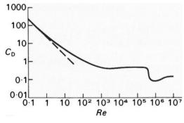
**Figure 1.**  $C_D$  vs. Re for a sphere. The dashed curve represents theoretical results for small values of Re [22].
